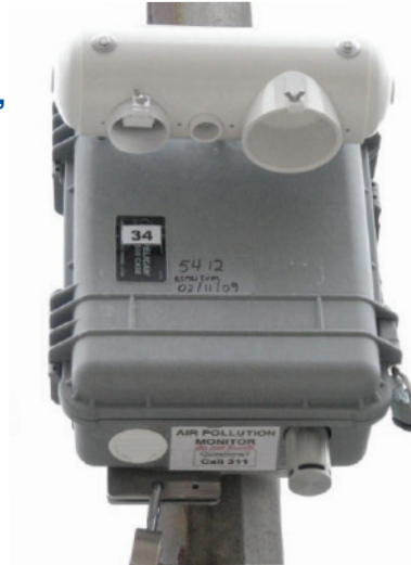
Figure 1. The New York City Community Air Survey uses portable air samplers mounted 10 to 12 feet from the ground on light poles, close to street level, to collect air samples throughout the 5 boroughs.
