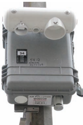
Figure 2. New York City Community Air Survey portable air sampler.
